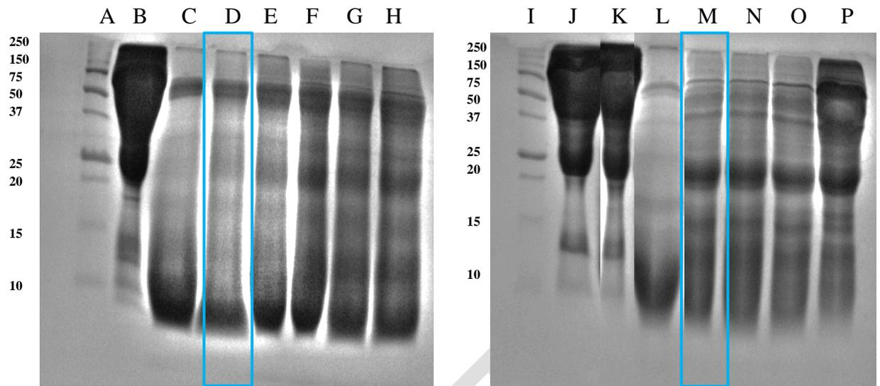
Figure 2: 15% SDS-PAGE of cattle and goat blood plasma hydrolyzed with Thermolysin from *Geobacillus stearothermophilus* (pH 7.5/ 37°C). Lane A and I = Marker, Lane B= Cattle blood plasma, Lane C to H= Cattle blood plasma hydrolyzed at 37°C for 0, 3, 6, 9, 12, and 24 h, Lane J= Goat blood Plasma, Lane K to P= Goat blood plasma hydrolyzed at 37°C for 0, 3, 6, 9, 12 and 24 h.
